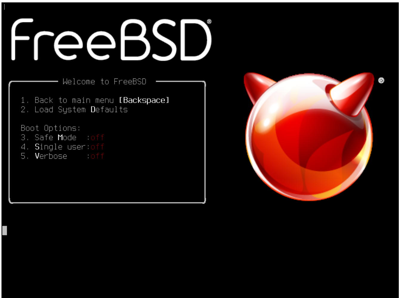
Figure 2. FreeBSD Boot Options Menu
